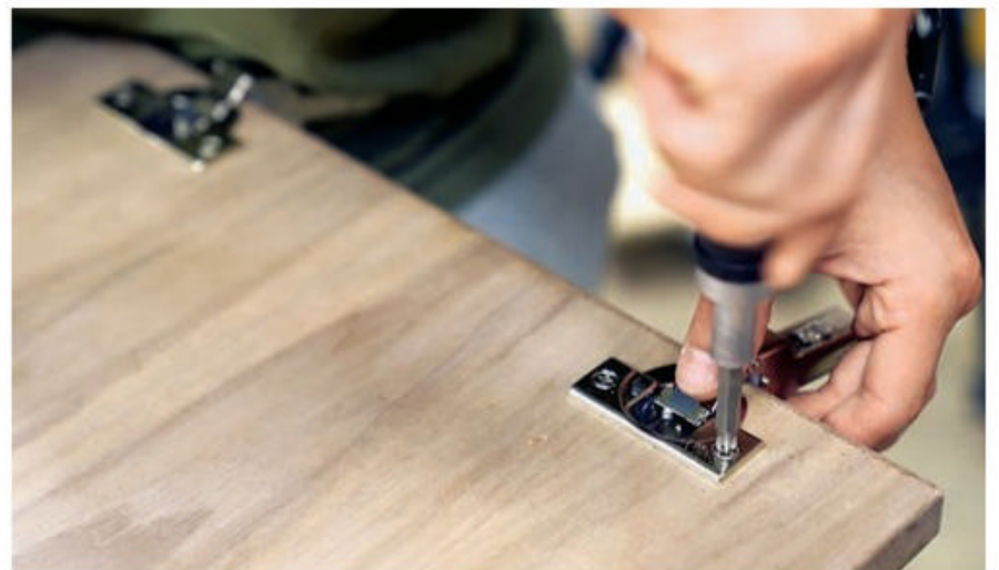
Insert the cup-side hinge components into their mortises in the door, and attach the hardware with screws. Make sure the hinge arms are square to the door edges before driving the screws.
