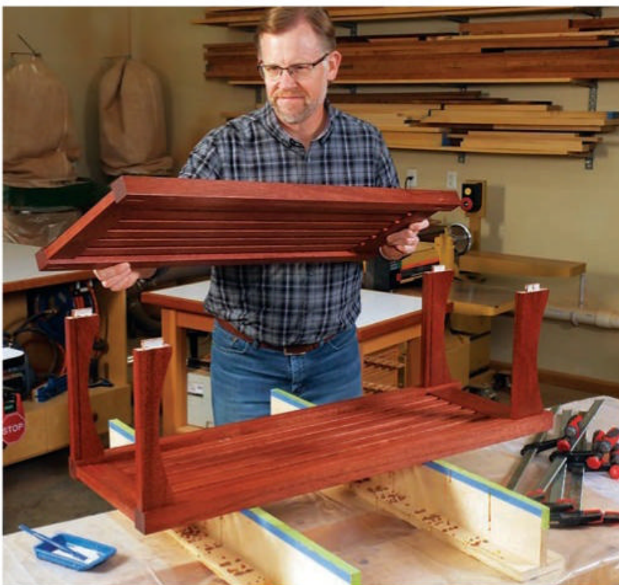
Sand, stain and topcoat the arched rails, then go ahead and bring the center unit together with glue and clamps.
