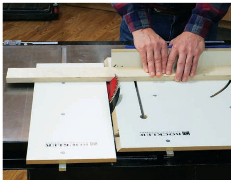
Crosscutting (here using a crosscut sled to make a 45-degree angled cut) is one of the two primary cuts performed by a table saw. A crosscut sled helps to make crosscutting safer and can add functionality.
