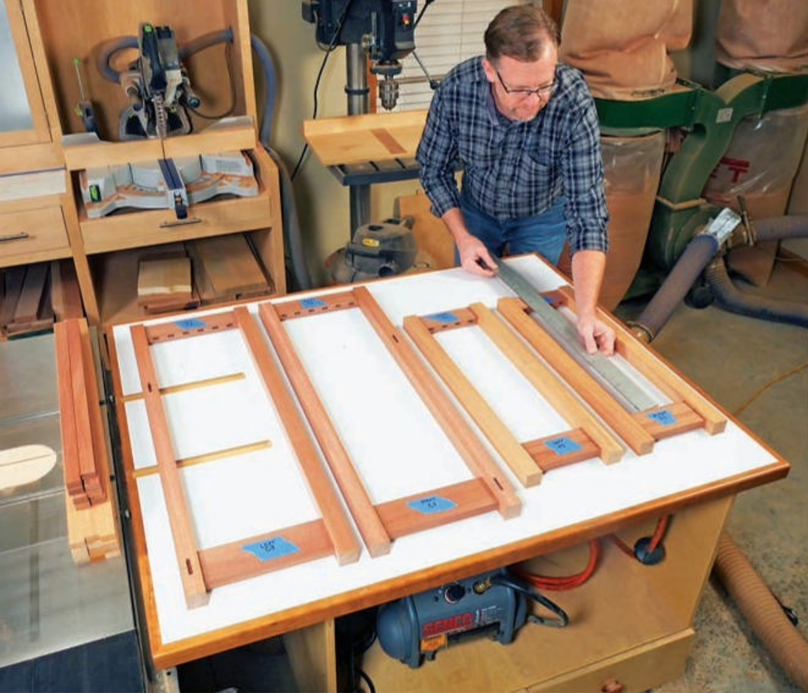
Dry-fit the side rails and legs of the center and outer units together into four frameworks so you can verify the slat lengths you'll need. The distance between the inside edges of the top and bottom rails, plus 1", equals the actual slat lengths.
