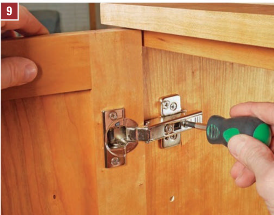
9 Use the hinges' adjustment screws to fine-tune door placement on the cabinet opening. Depending on the hinge, these screws provide very helpful up/down, side-to-side and in/out door adjustability.
