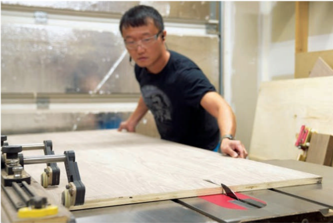
Break down 3/4" plywood to create panels for the top, bottom and sides of the carcass. Whether you use a table saw, circular saw and straightedge guide or a track saw and track, be sure to install a sharp blade to cut the walnut veneer cleanly. It's most liable to splinter across the grain.
