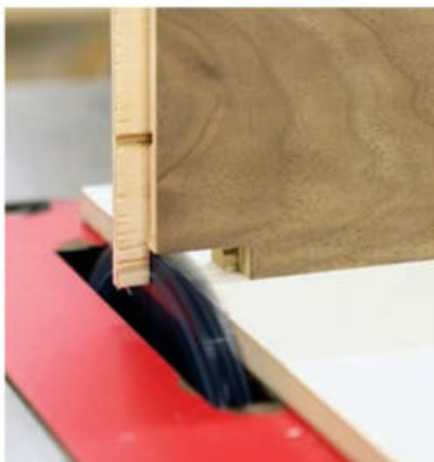
Mill 1/2"-wide, 1/4"-deep rabbets into the ends of the inside faces of the drawer side panels. The author used a wide dado blade for this task.
