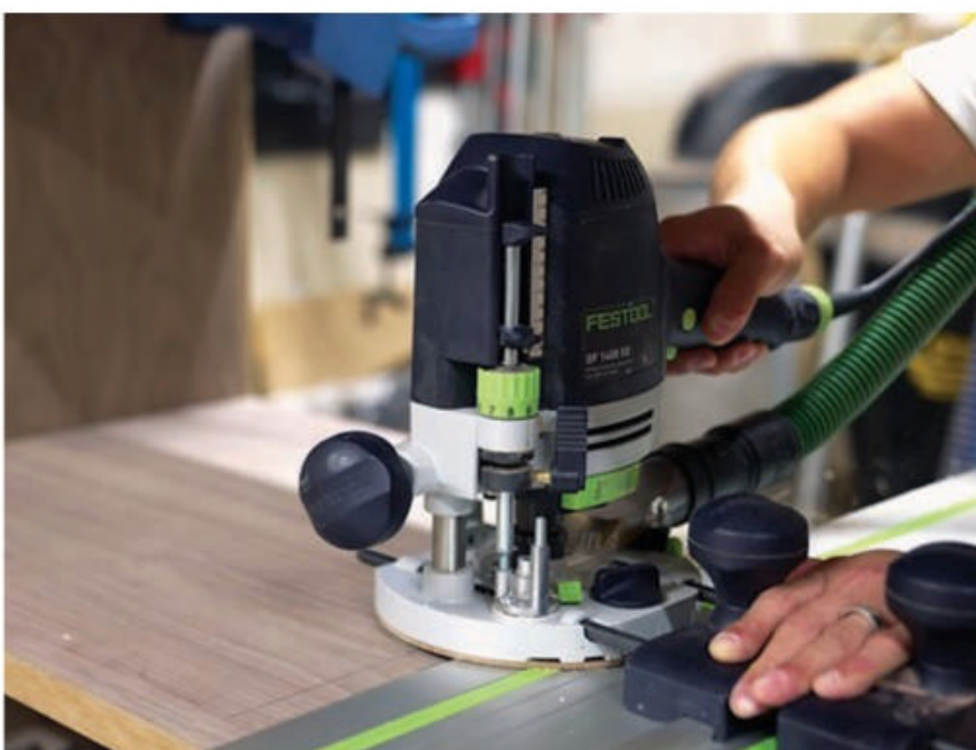
Mark the shelf to locate dadoes for the small upper and lower vertical partitions, and plow these 1/4"-deep stopped dadoes into it.
