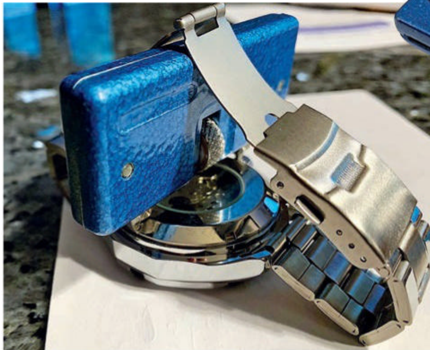
Vince Piacenti's watch crab closely resembles Paul Doman's October mystery tool. Here, its jaws are engaged in the notches of a watch back. Twisting the tool right or left threads the back on or off for repairs.
