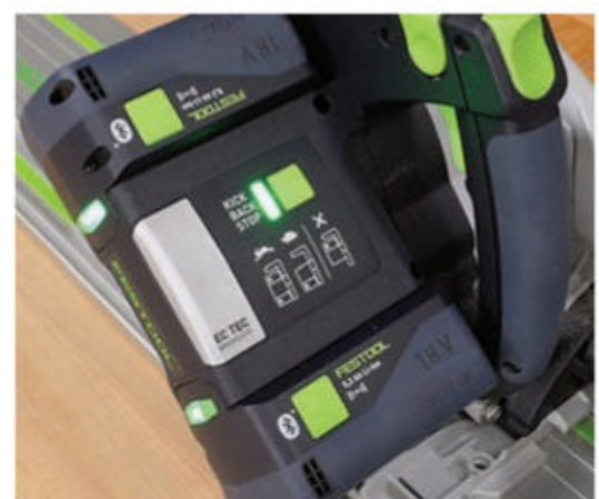
The anti-kickback feature can be controlled by a button on the left side panel of the saw. It can be turned off completely or adjusted to fast or slow.
