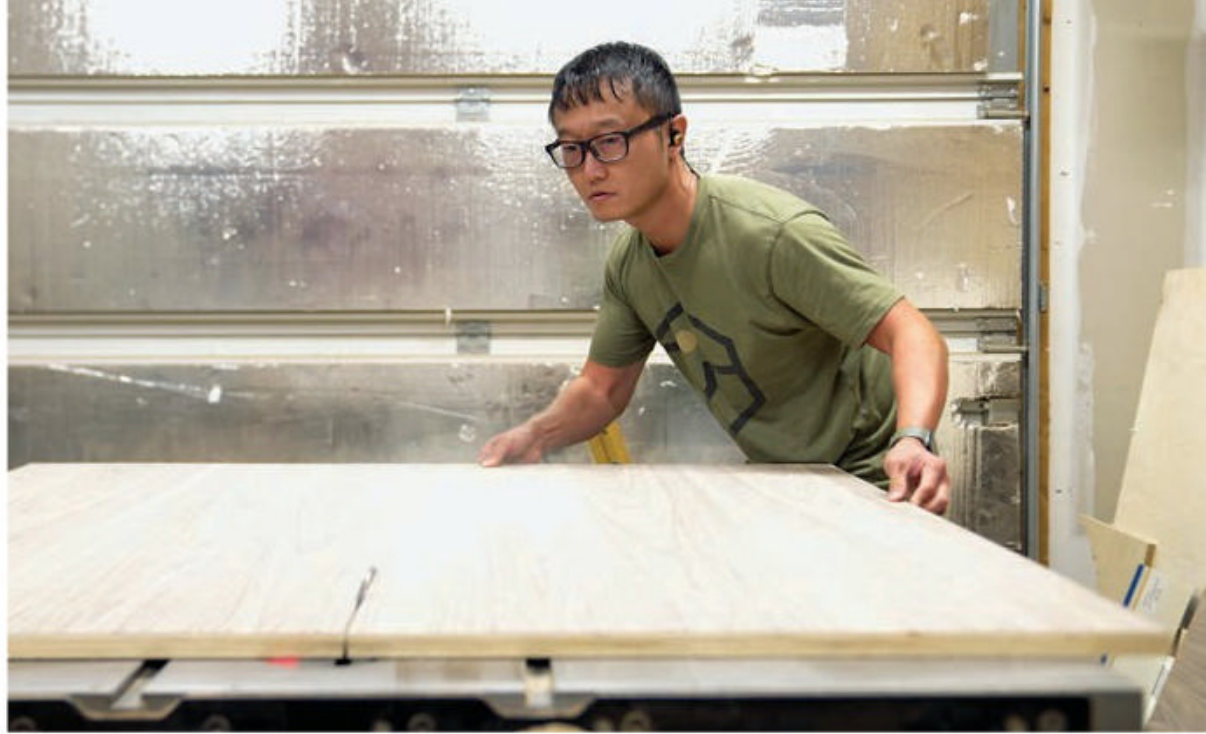
Cut 3/4" plywood to size for the two door panels. Be sure to take into account the thickness of the edge banding you'll be adding around their perimeters as well as the gaps the doors will require in their carcass openings.
