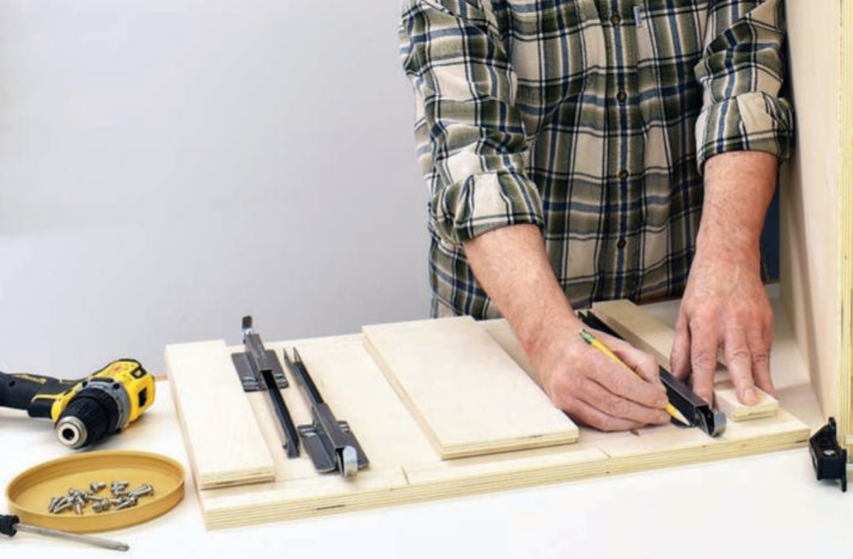
Before assembling the cabinet carcass, use the three sub-tops to lay out and mark locations for the leaf support brackets on the underside of the main top. Then mark the exit hole locations of this hardware on the cabinet sides.
