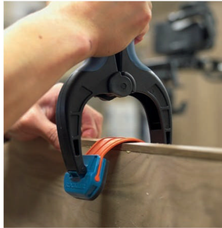
The author glued 1/8"-thick banding to every part edge where the plys would show. Rockler's Bandy Clamps are handy for holding this edging in place.
