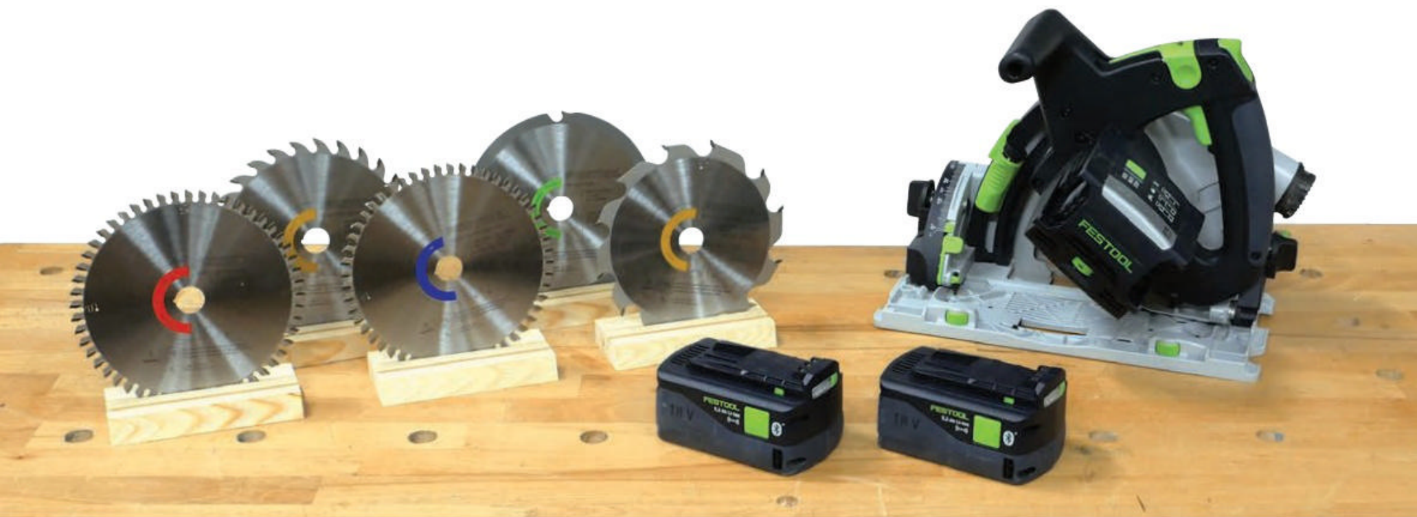
The new TSC 55 K can be used with a full complement of thin-kerf saw blades. Color-coded, three of them are for specific woodcutting uses. Another is for high-pressure laminate or aluminum and a fourth blade is for concrete. Thin-kerf geometry helps the 18-volt batteries deliver more cuts per charge.
