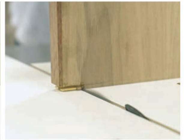
While the Material List provides the length of the large vertical partition, it's always a good idea to measure off of your actual project (left) to verify captured part lengths like these. Once it's cut to size, notch the front corners of the partition so it fits into and around the carcass dadoes (center, right photos). All three of the carcass's partitions and horizontal shelf will be notched this way.
