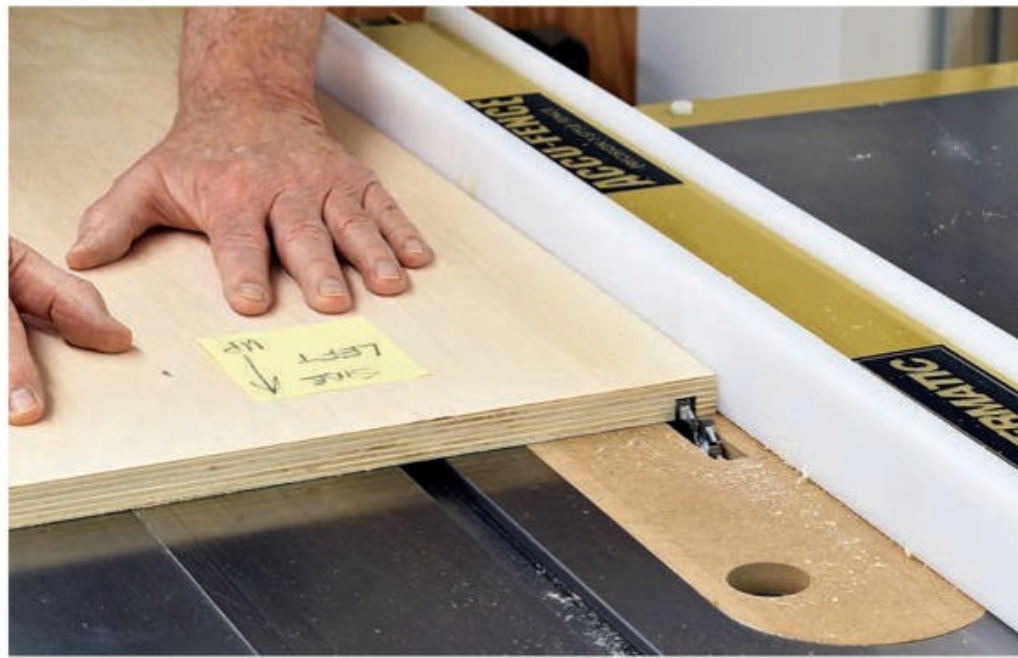
Make all the needed rabbets and dados for the workpieces on the table saw with a dado cutter, as shown here, or using a router table equipped with a straight or spiral bit.
