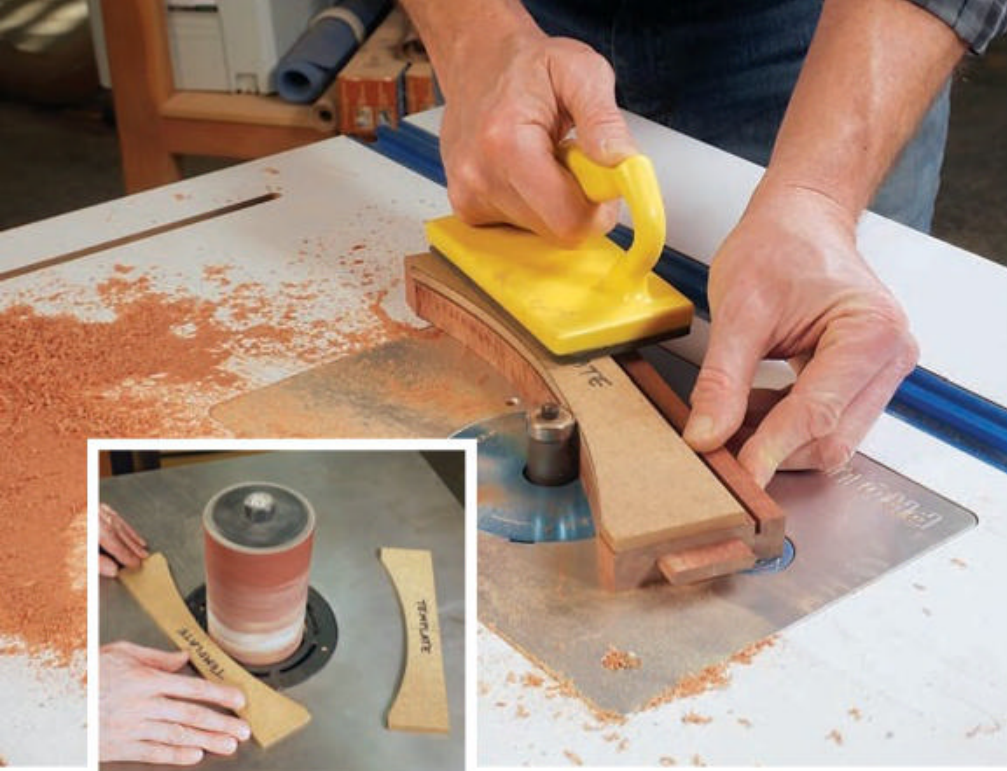
The author made a pair of rail templates from 1/4" scrap MDF (inset) to ensure that the arches on the front and back rails would be uniform. He used them for both tracing the curves and template-routing the actual parts.
