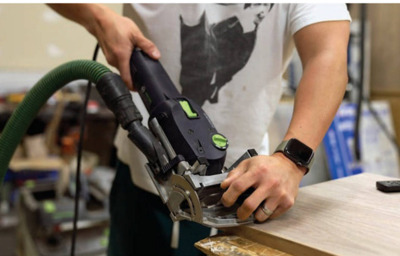
Long bevel joints like these will be very difficult to keep aligned during glue-up unless you reinforce them with loose tenons or biscuits. These reinforcements also strengthen the carcass joints.
