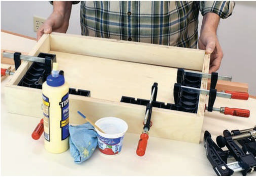
Glue and clamp the drawer box components together, being careful to keep the assembly square. Repeat the process with the pullout shelf.
