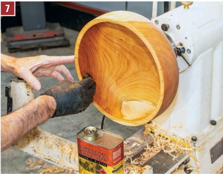
7 Apply the first coat of finish to the inside. The author is using Waterlox Original Sealer Finish, but mineral oil, walnut oil or various "salad bowl" finishes would be other good choices, too.
