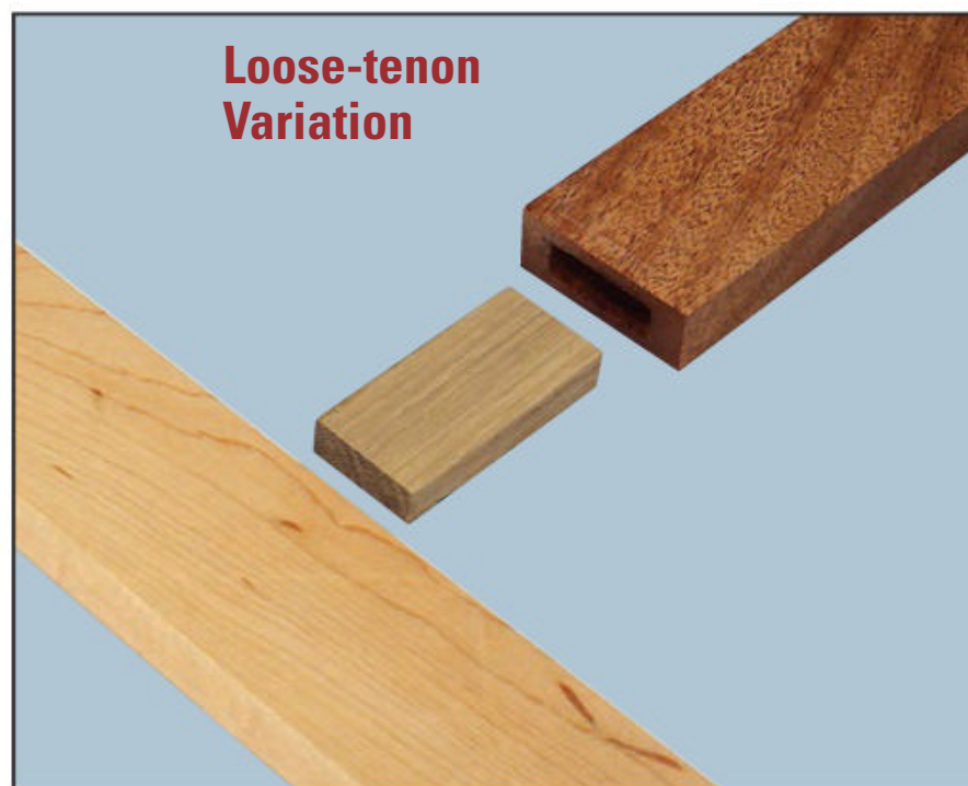
A tenon doesn't have to be machined onto the end of one joint member; it also can be a third, separate element, bridging both workpieces and fitting into matching mortises in the parts.
