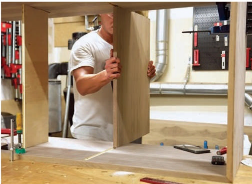
Slide the vertical partition into place and mark it for a horizontal shelf dado. The author installed a temporary plywood brace between the top and bottom panels to correct for slight sagging of the top panel.
