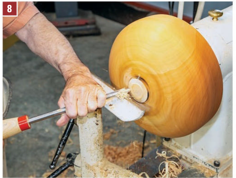
8 Reverse the bowl onto either a jam chuck or a vacuum chuck. Turn the bottom to a very uniform, convex shape, and bring the wall of the bowl to a constant thickness from the rim to the center of the base.
