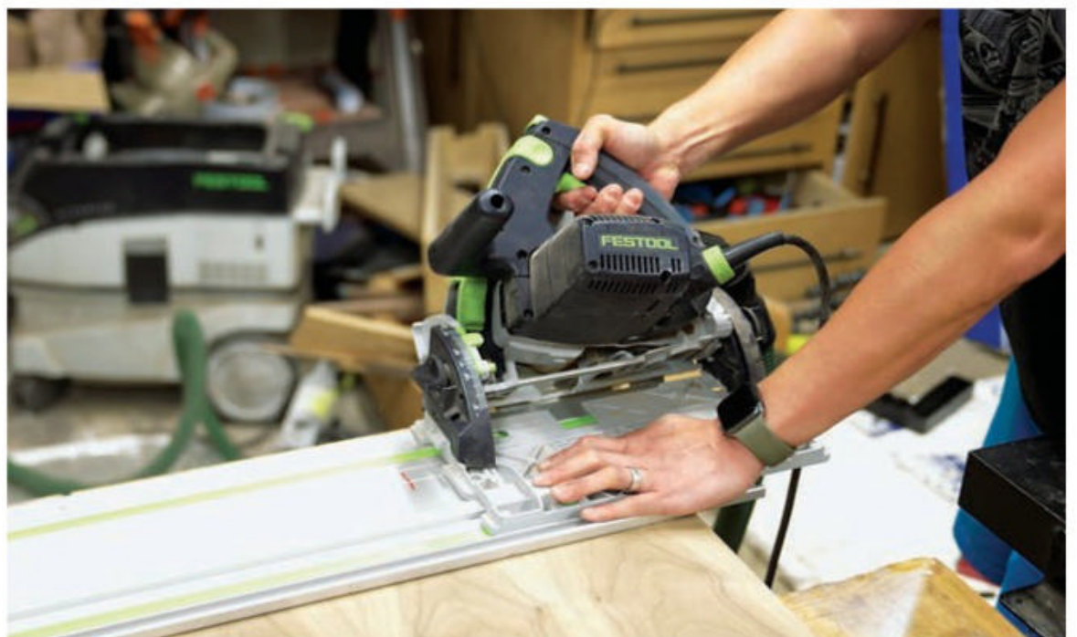
Bevel-cutting the ends of the top, bottom and side panels will be easiest to do with a track saw tilted to 45 degrees. If you don't have a track saw, a conventional circular saw, guided along a clamped straightedge, will also work for this operation. Make these cuts slowly and carefully,
