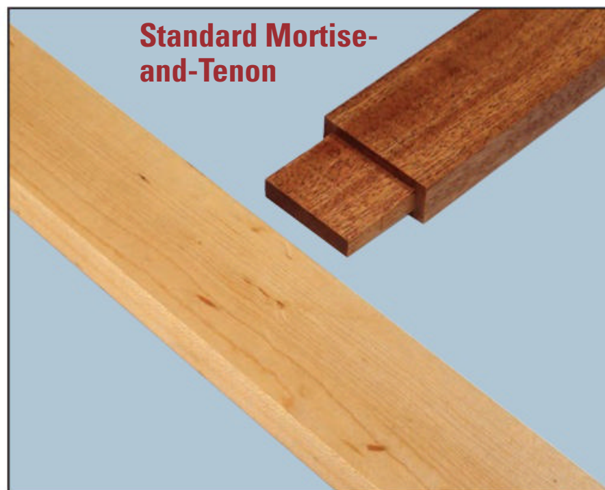
On typical mortise-and-tenon joints, the protruding tenon fits into a squared and matching excavation in the mating part, called a mortise. Once assembled, all visible evidence of the joint is hidden.
