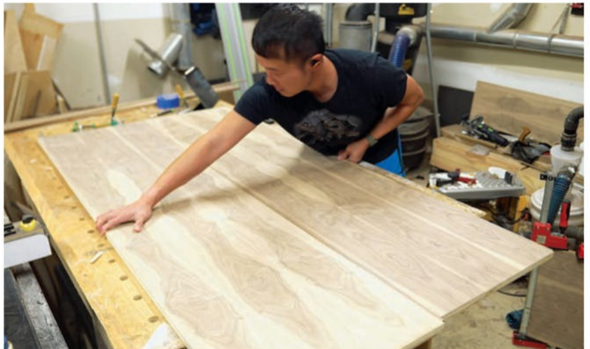
Set the top and bottom panels together with their ends aligned to prepare for bevel-cutting their ends. Gang-cutting them this way will ensure that the panel lengths remain the same.
