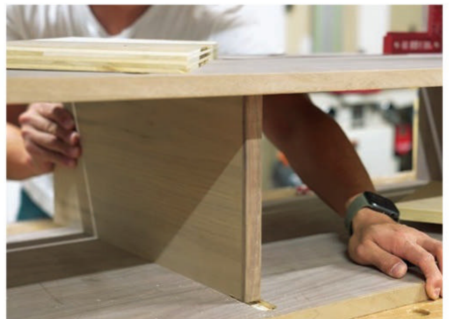
Again, measure between the dadoes in the shelf and top and bottom carcass panels to determine the small vertical partition sizes. Once you've cut, banded and notched them, check their fit in the carcass.
