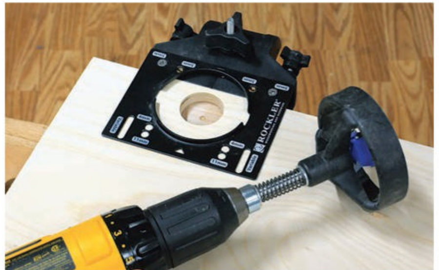
A cabinet door drilling jig paired with a 35 mm Forstner bit makes quick work of boring the mounting cup holes for Euro-style hinges.
