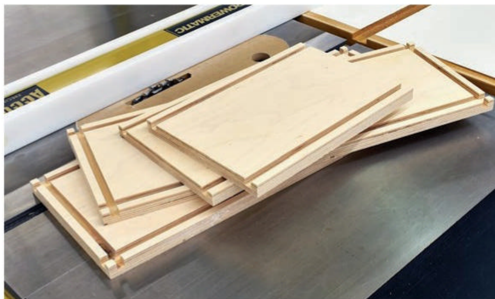
The author mills dados and rabbets first, then cuts the workpieces to final width when making particularly narrow parts. It's safer and more efficient.
