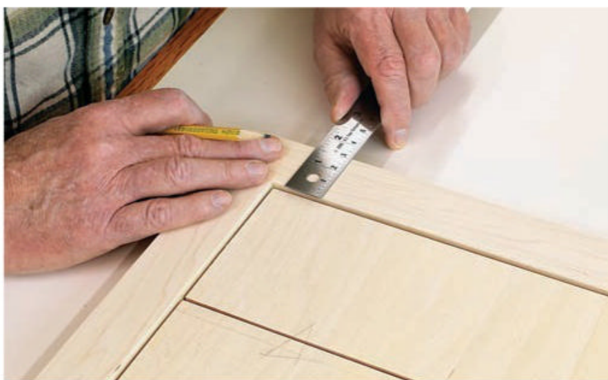
Another task best done before attaching the face frame to the cabinet is checking and tweaking the fit of the door and drawer face. A gap of about 1/8" all around is fairly standard and looks good.
