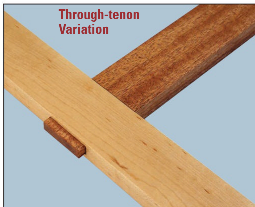
Sometimes an elongated tenon passes all the way through the mortised workpiece so its end extends beyond the other edge. This decorative treatment often appears on Arts & Crafts furniture.
