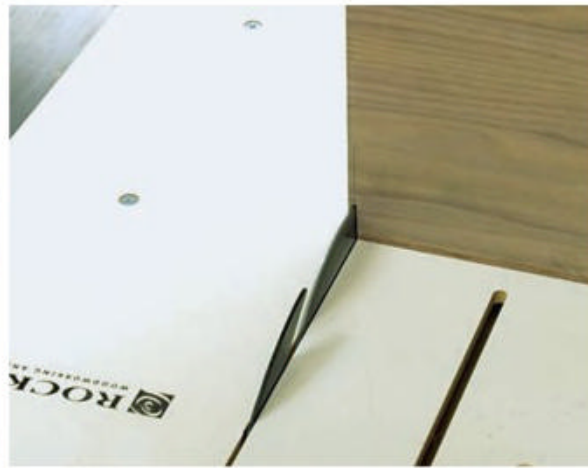
While the Material List provides the length of the large vertical partition, it's always a good idea to measure off of your actual project (left) to verify captured part lengths like these. Once it's cut to size, notch the front corners of the partition so it fits into and around the carcass dadoes (center, right photos). All three of the carcass's partitions and horizontal shelf will be notched this way.
