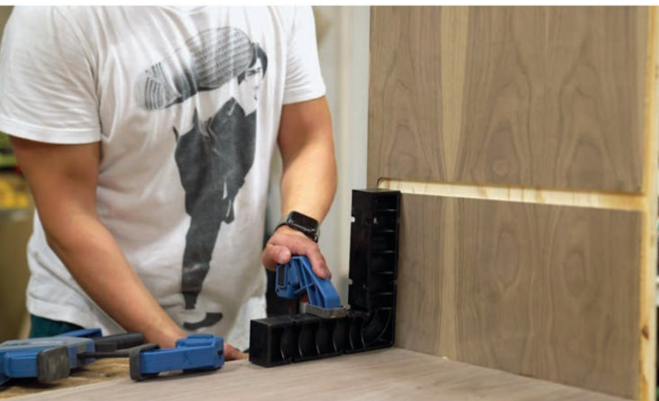
Long bevel joints like these will be very difficult to keep aligned during glue-up unless you reinforce them with loose tenons or biscuits. These reinforcements also strengthen the carcass joints.
